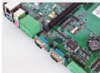
8KV ESD, TVS 600W Surge Protection for COM port
