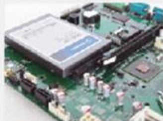
Direct HDD connection No internal cabling
