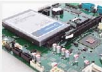
Direct HDD connection No internal cabling
